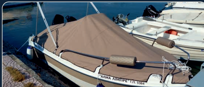
Mooring cover (Sunbrella fabric, Inox 316 safety clips)
